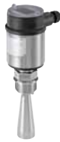
Radar fill level transmitter 8137 for general high-pressure applications, compact transmitter for fill level measurement up to 30m, 4...20 mA / 20 mA / Hart – 2 wires, ATEX Cat.1/2G
