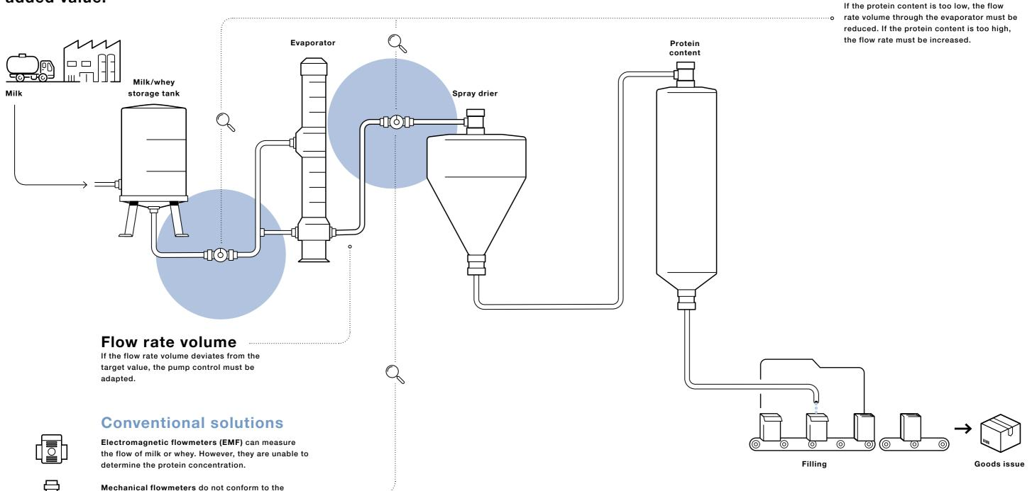
/ Flow measurement with SAW technology / Hygiene is particularly important during the production of dairy products. FLOWave gives you a compact solution that measures the flow under completely hygienic conditions. Thanks to innovative SAW technology, the flowmeter dispenses with sensor elements in the measuring tube. No parts in the measuring tube means: no deposits, no material incompatibility, no maintenance, no pressure drop and easy cleaning.
